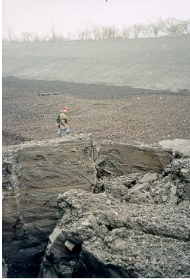
Geologist on failed landslide block along western high wall of landfill.
