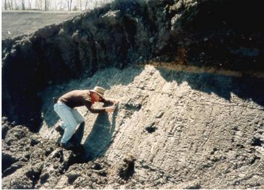
Geologist performing fracture orientation measurement along landslide scarp on failed western wall of landfill.
