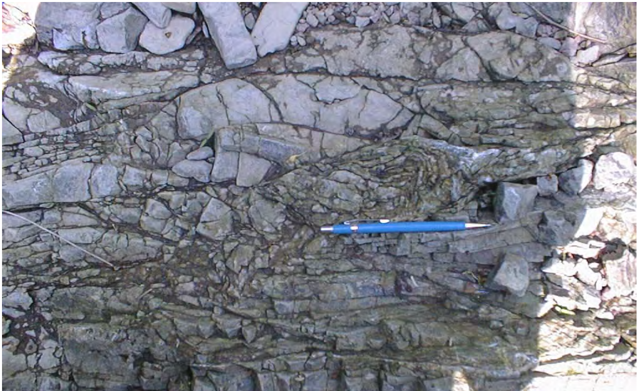
Shear fabric within Orange Mt. basalt in the Flemington fault zone.
