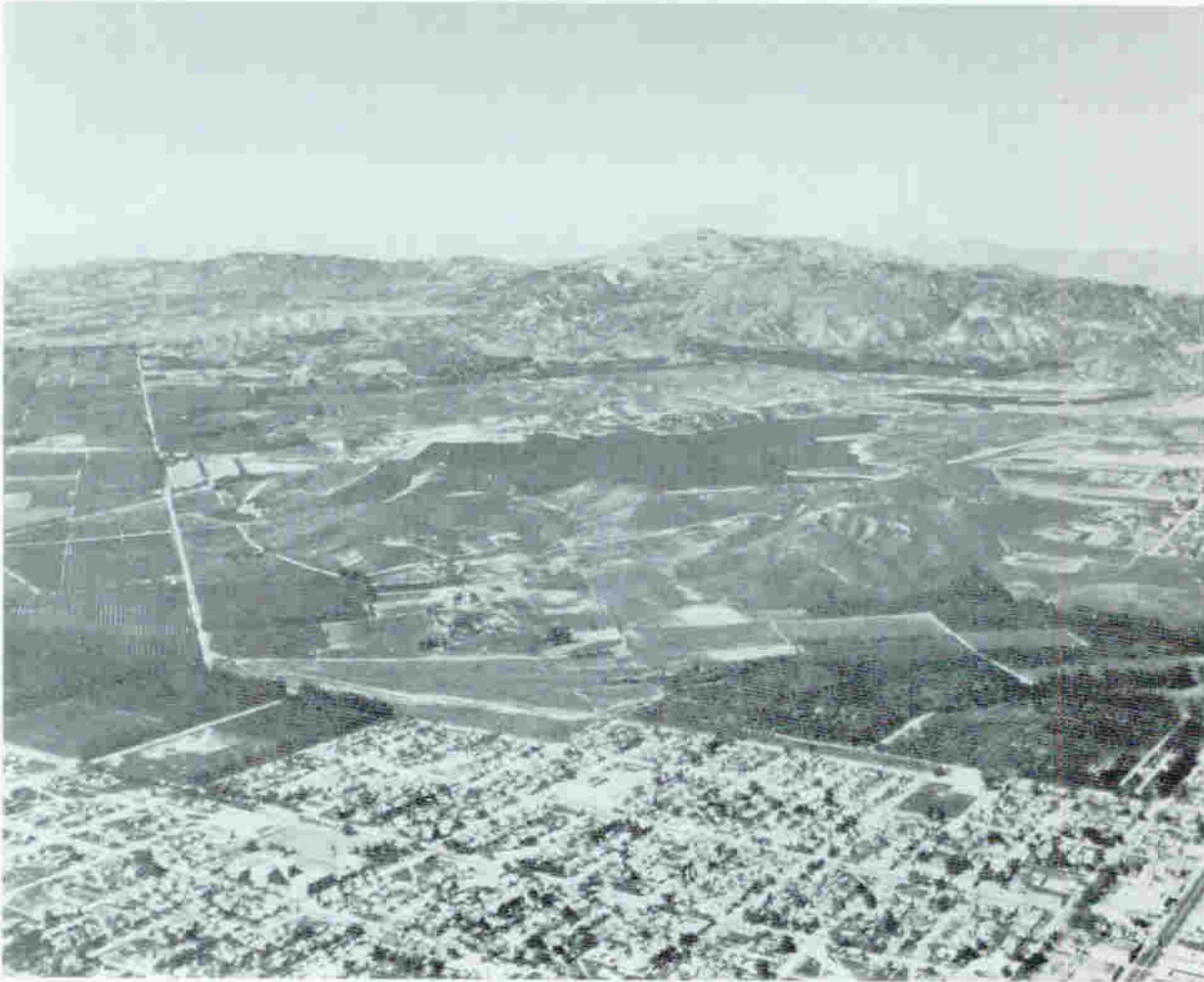
Figure 5. The Lower Van Norman Reservoir (center) and smaller Upper Van Norman Reservoir (right) in the northern San Fernando Valley, as they appeared in 1950 before nearly all of the downstream area at left had been developed for residential purposes. Rupture and gross displacements occurred in both of the dams during the San Fernando earthquake of February 9, 1971, endangering tens of thousands of people in the thickly settled downstream area. Pacific Air Industries photograph.
