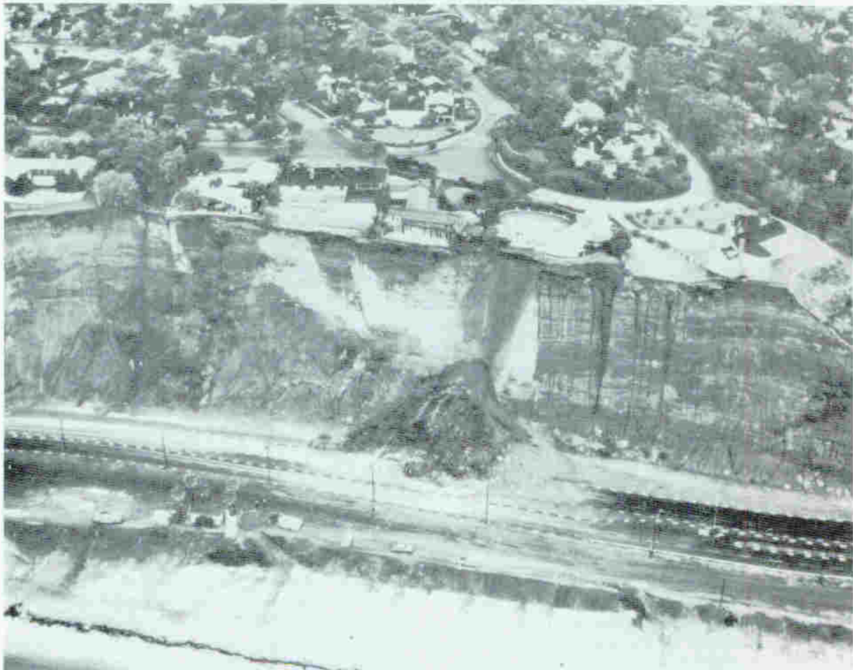
Figure 9. Local detachment and collapse of cliff-forming alluvial deposits along the coastline at Pacific Palisades, November 1966. Clearly visible in this view is evidence of earlier encroachments on the residential area above the cliff, Pacific Air Industries photograph.
