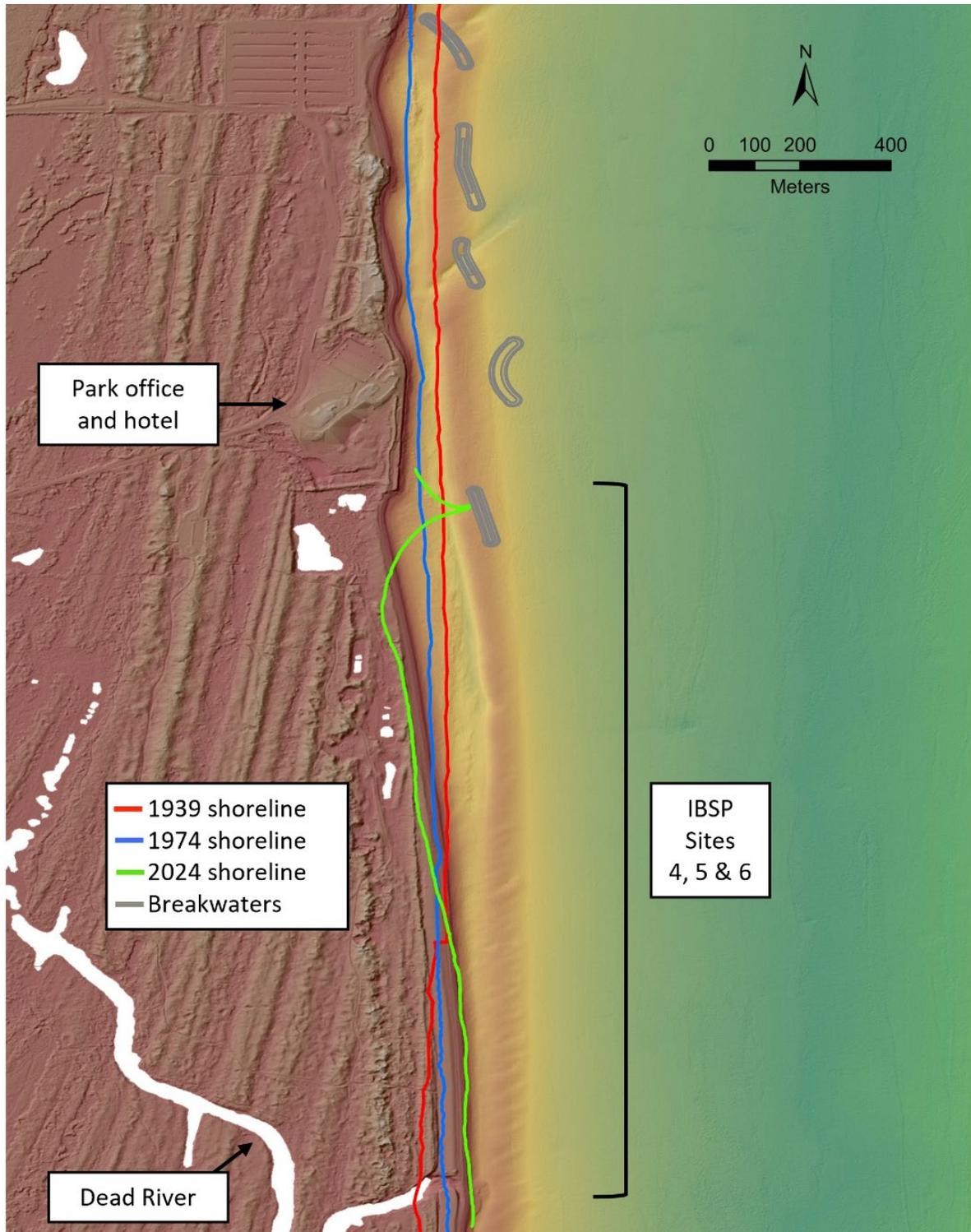
**Figure 32** – Hillshaded DEM based on 2020 LiDAR data depicting the once continuous nearshore sandbar, where now a series of emergent breakwaters exists (since 2023). The nodal point separating historically erosional from depositional parts of the ZBRP occurred between the IBSP hotel and the Dead River, near where 1939 and 1974 shoreline positions cross.
