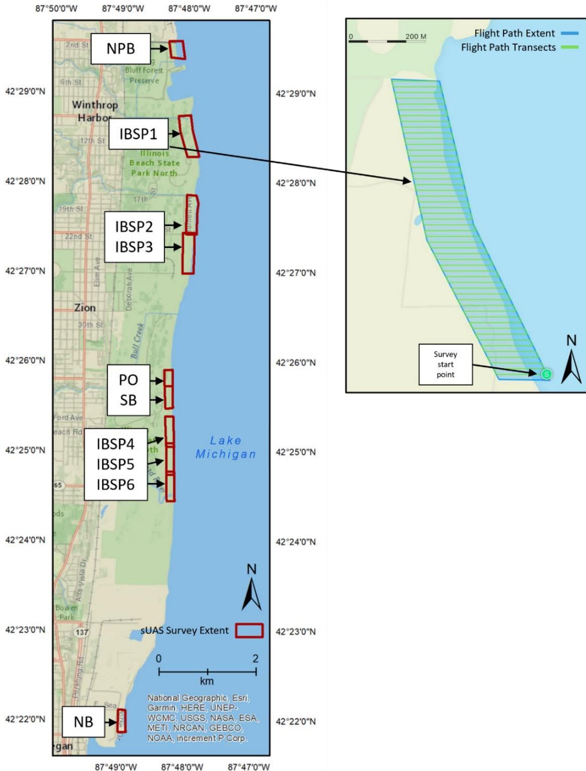
**Figure 18** – Map of the Illinois portion of the ZBRP showing ISGS shoreline-monitoring locations, along with an inset map depicting the aerial drone (UAS) flightlines for image acquisition (for Structure from Motion Photogrammetry and DEM creation).
