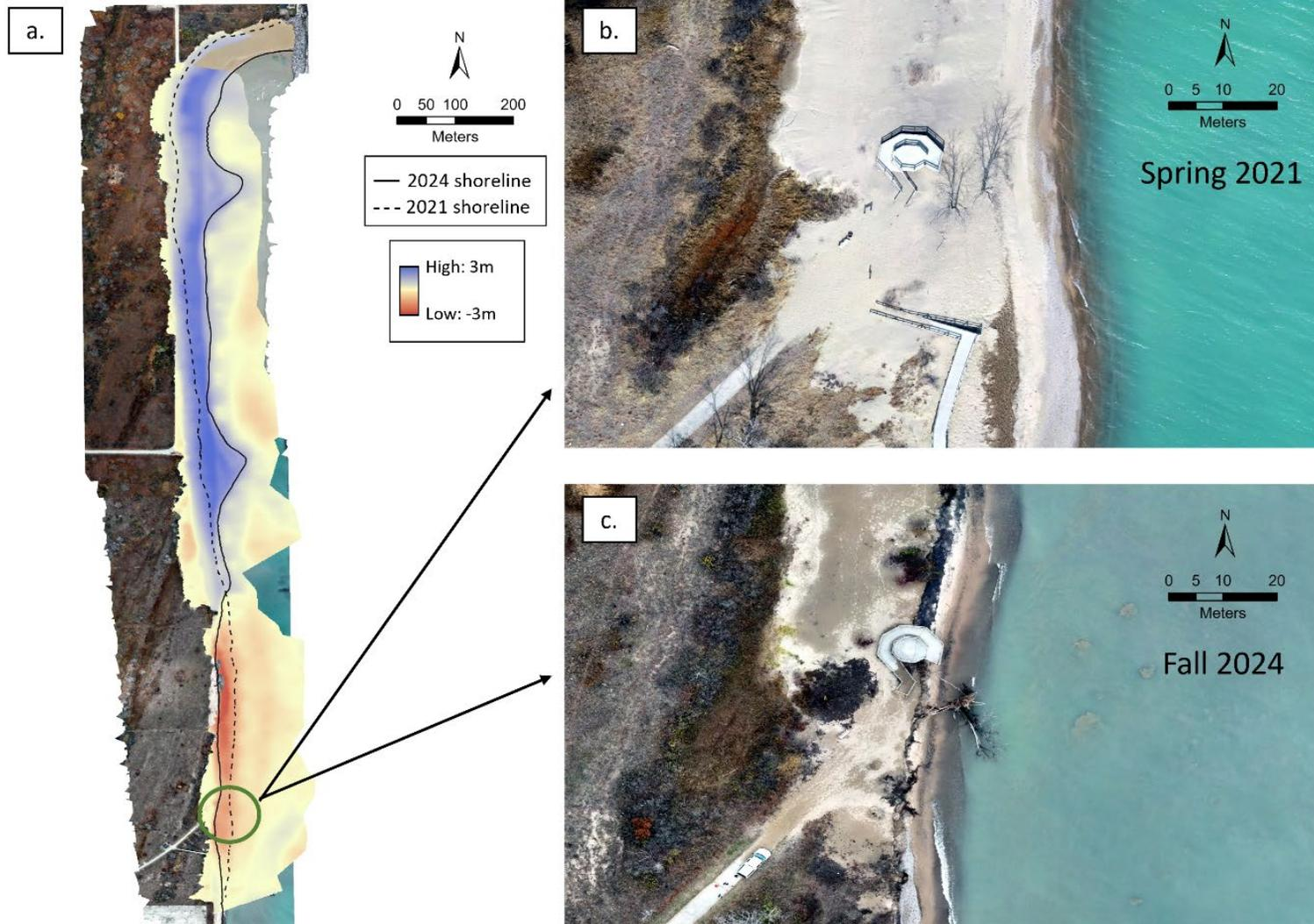
**Figure 30** – Net change model for 2021-2024, with inset photographs from spring 2021 and fall 2024 that capture the demise of lakefront viewing platform and boardwalk. This area had not yet been impacted when lake level was rising, from 2012 to 2020, but began eroding more heavily with lake-level fall (especially once breakwaters had been built to the north).
