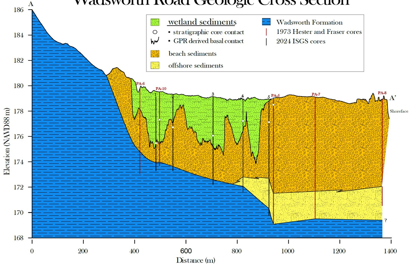
**Figure 14** – Geologic cross section of Wadsworth Road, constructed from 2024 ISGS Geoprobe cores and archival information from 1970s stratigraphic assessments by Hester and Fraser (1973). The location of this cross section is Wadsworth Road, from bluff to shoreline, as shown in Figure 1b.
