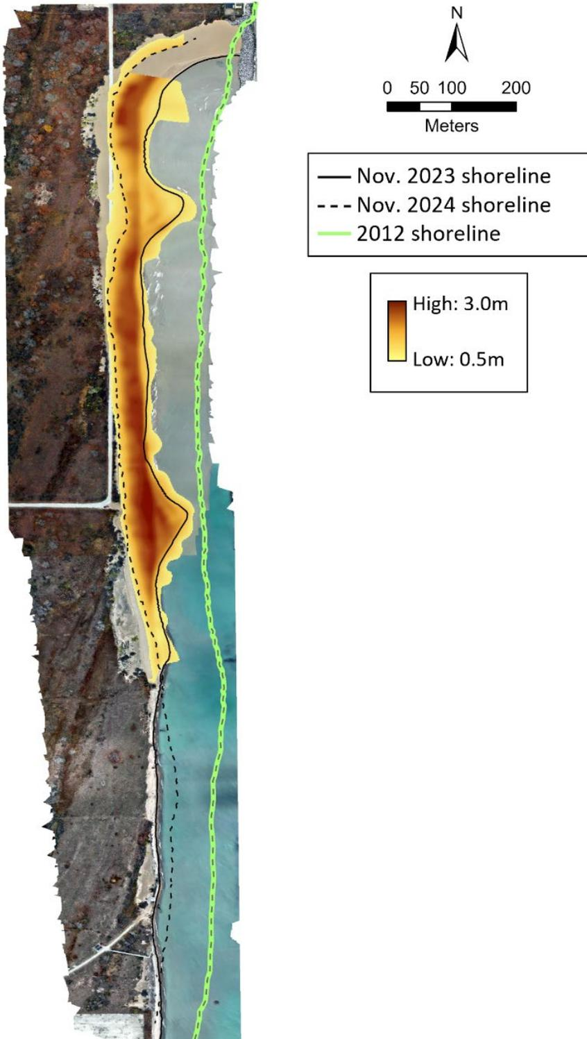
**Figure 29** – Sand isopach model for what was placed, as part of 2023-2024 breakwater construction and beach replenishment efforts. Total volume approximates 89,364 m<sup>3</sup>.
