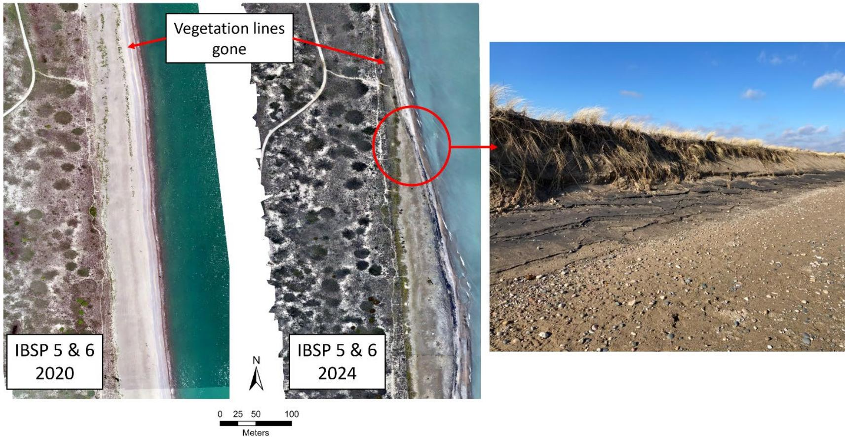
**Figure 34** – Orthoimages from 2020 and 2024 showing developments along the approximate nodal zone between IBSP4 and IBSP6, where recently accreted foredune terrains are now being truncated by shoreline retreat. A 2-meter berm extends along much of this section of shoreline today, with thick heavy mineral placer deposits occurring at the base of the scarp (from reworking of eroded sediments by swash processes).
