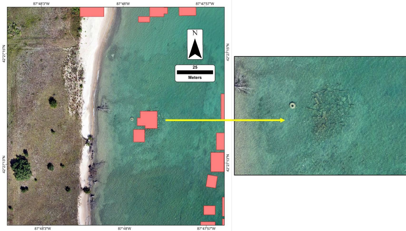
**Figure 9** – ISGS CGG-derived orthomosaic based on drone imagery from September 12<sup>th</sup>, 2024. It is overlain by a polygon layer of historical home locations. An enlarged portion of the image is shown to the right. With a net-export of sand from these shoreline regions, the former infrastructure remains visible on the lake bottom. It is imaged in sonar datasets and aerial drone imagery (on clear-water days).
