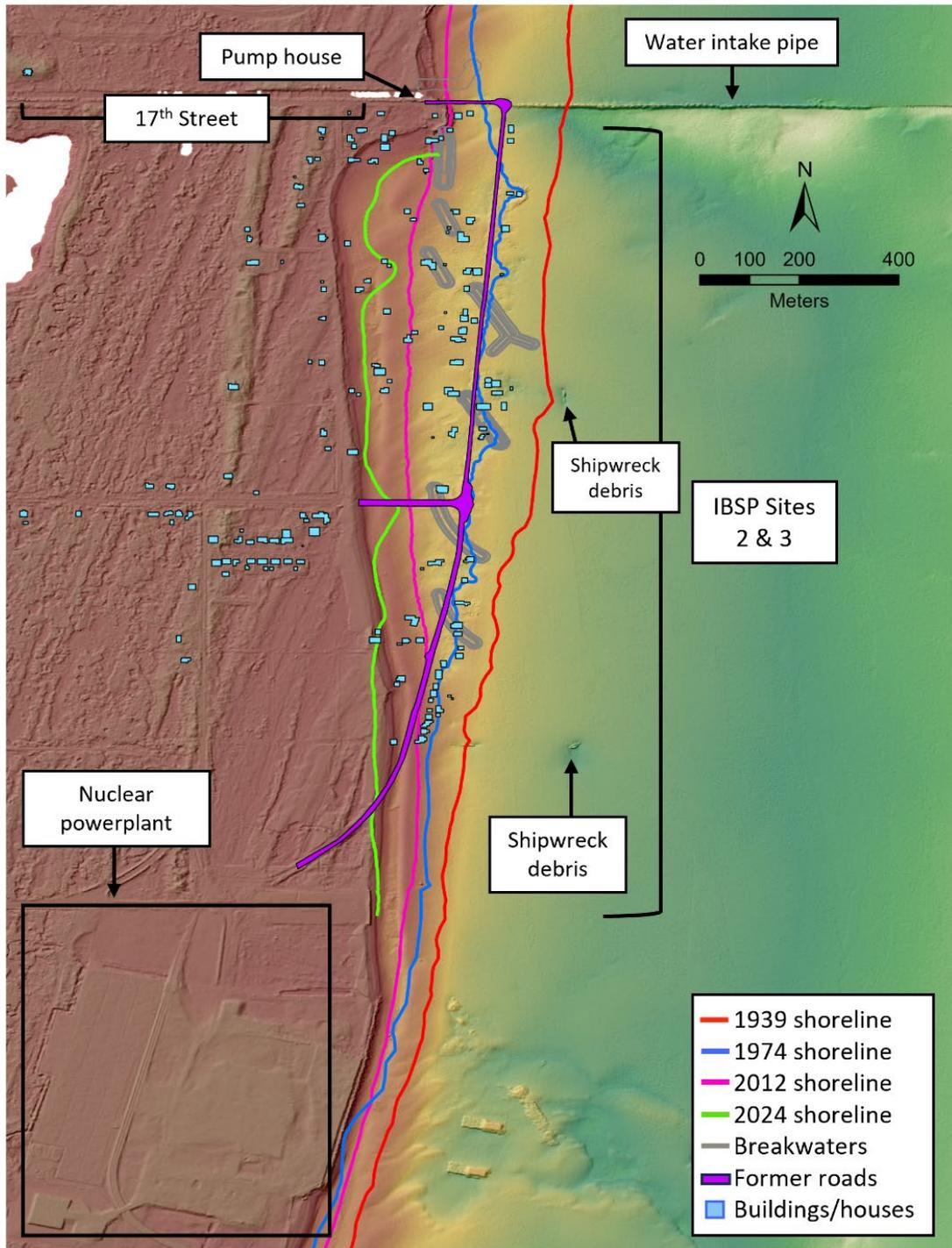
**Figure 27** – A map of IBSP 2 and 3 showing the houses (blue boxes) and roads (purple lines) that used to exist when the shoreline extended further lakeward in the 1970's. Notice the scour on the leeward side of a shore-perpendicular water-intake structure leading to the pumphouse on shore, just south of which erosion has been most severe.
