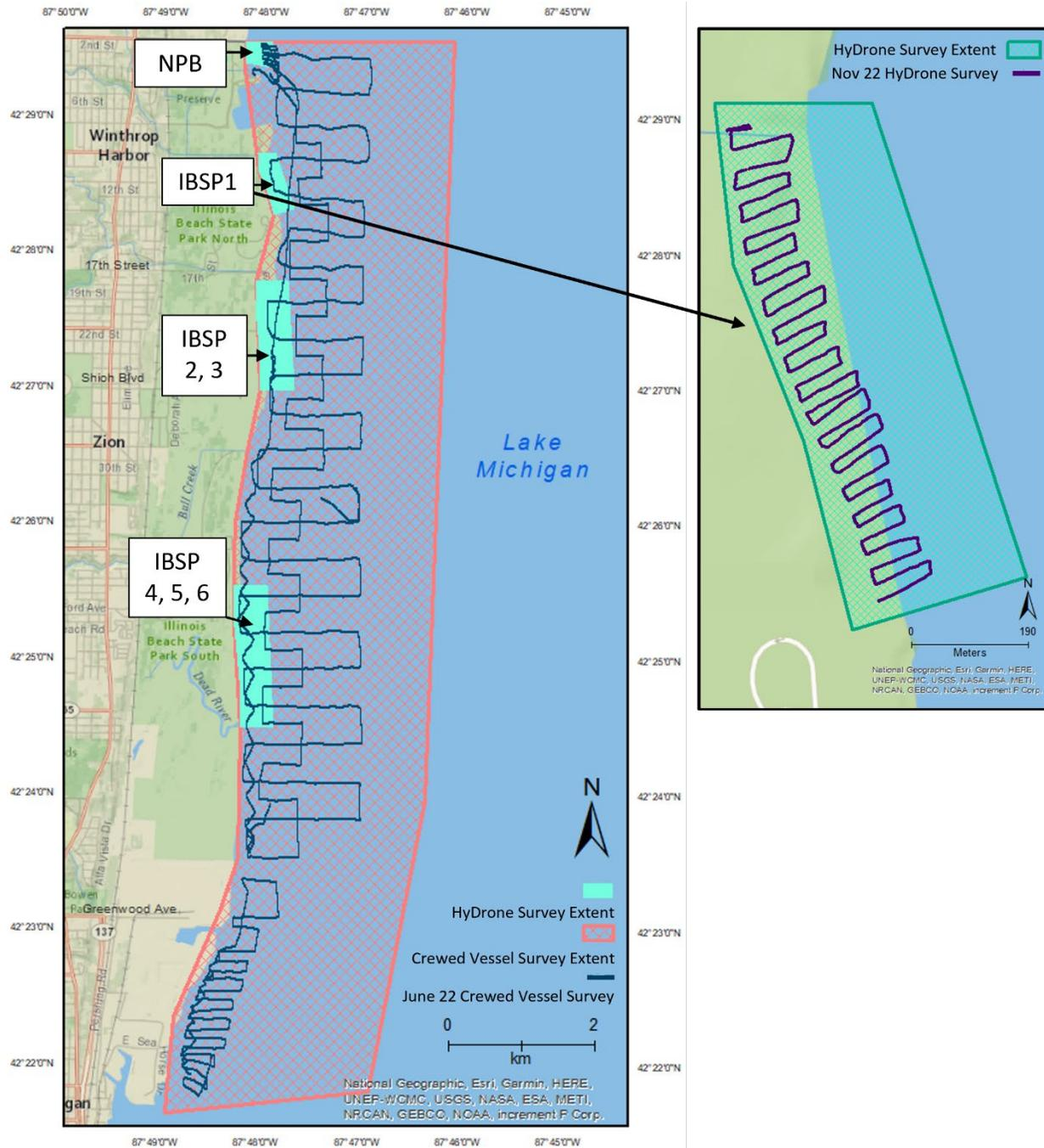
**Figure 19** – Map of the Illinois portion of the ZBRP showing a year's coverage of offshore sonar data, acquired close to shore using a remotely controlled vessel (see inset map) and across an offshore grid of 0.5 km spacing between shoreline-perpendicular transects using a crewed vessel. All surveys are single-beam sonar (SBES).
