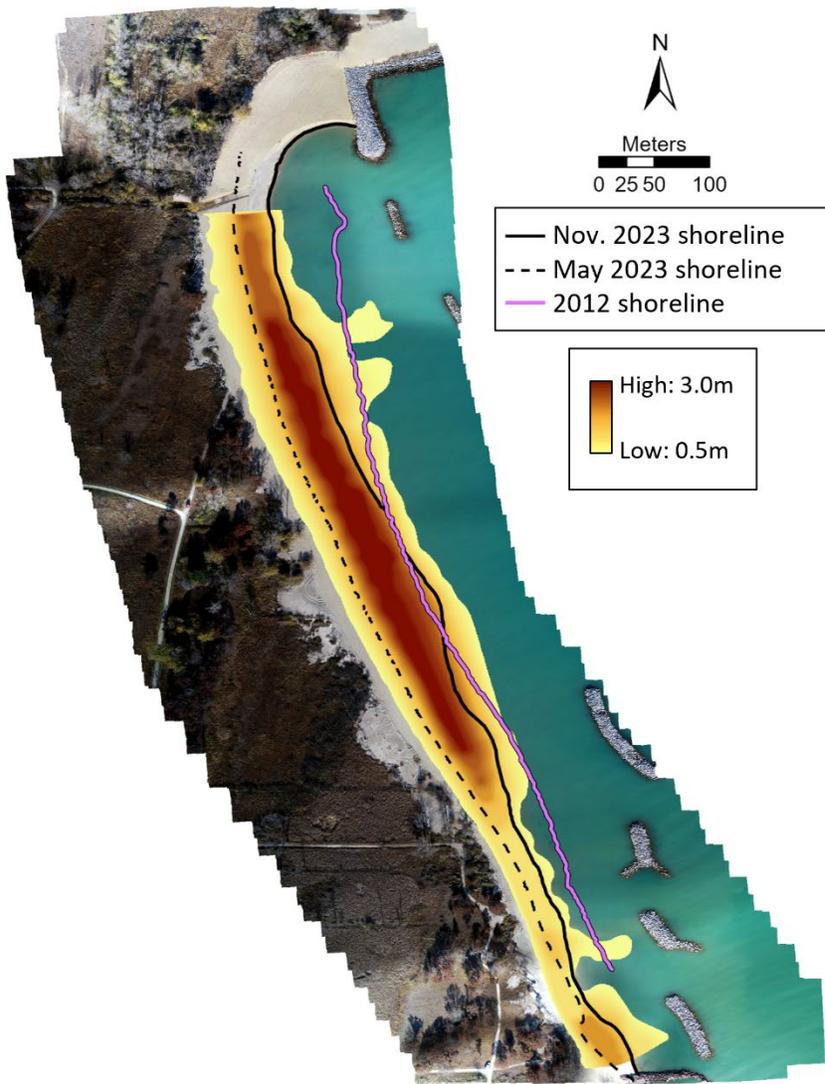
**Figure 25** – A net change map showing the amount of sand emplaced between May of 2023 and November 2023, alongside the construction of offshore emergent breakwaters. Around 77,364 cubic meters of sand were replaced at this site. Nearly 20% less than the amount of sand lost to shoreline retreat from along this shoreline between 2012 and 2020.
