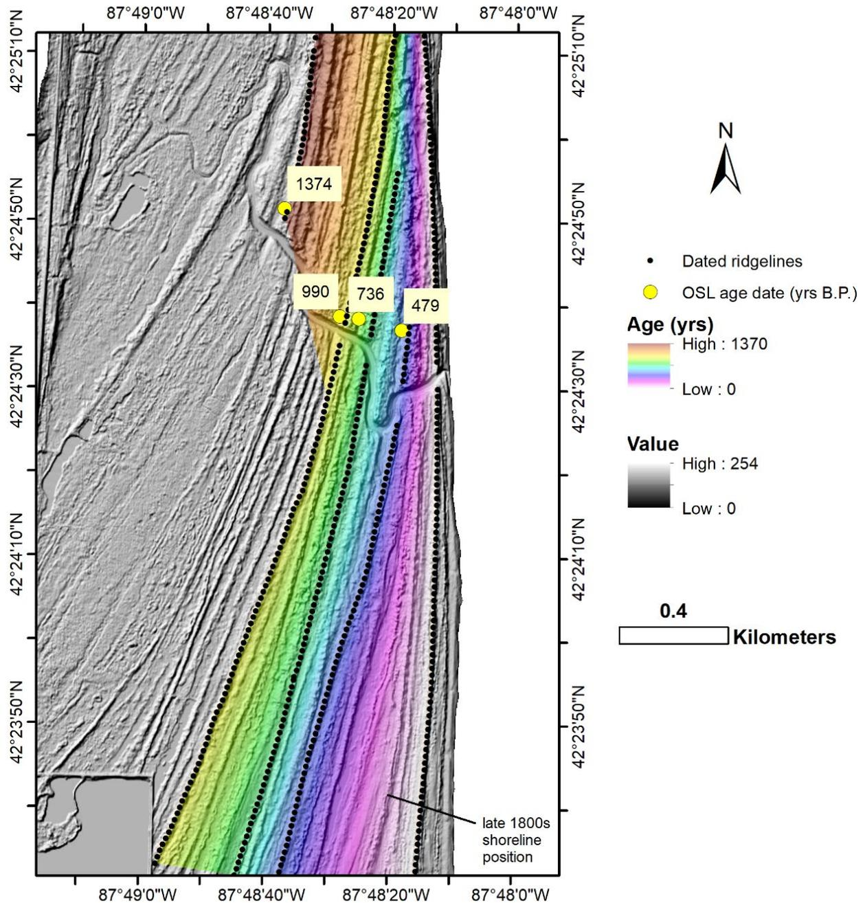
**Figure 13** – Hillshade map (5X VE) of the Dead River area (IBSP South Unit and southward) showing established OSL ages of ridgelines (dashed) cored for material to age date. The color-ramped surface is an interpolation of these ridgeline ages. There appears to be a more continuous chrono-sequence of ridges here than along the IBSP North Unit, where erosional truncation has visibly reworked portions of the ridge plain at different points in time (see Figure 12).
