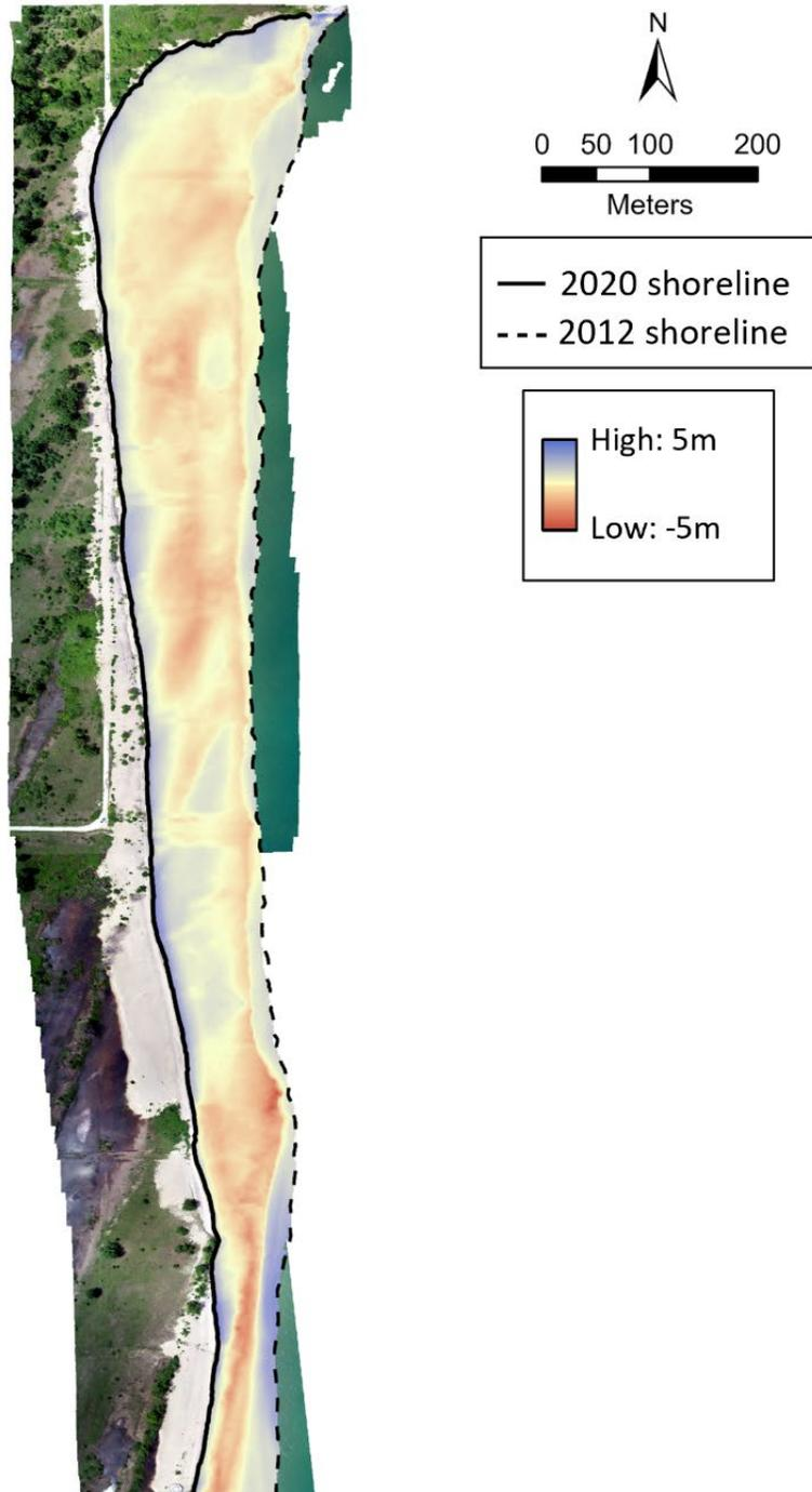
**Figure 28** – A geomorphic change model based on LiDAR bathymetry data from 2012 and 2020. Notice the lower erodibility of a shore-oblique beach ridge, which meets the shoreline in the lower part of the map, which separates areas of overwash accretion within swales and where the amount of shoreline retreat is reduced.
