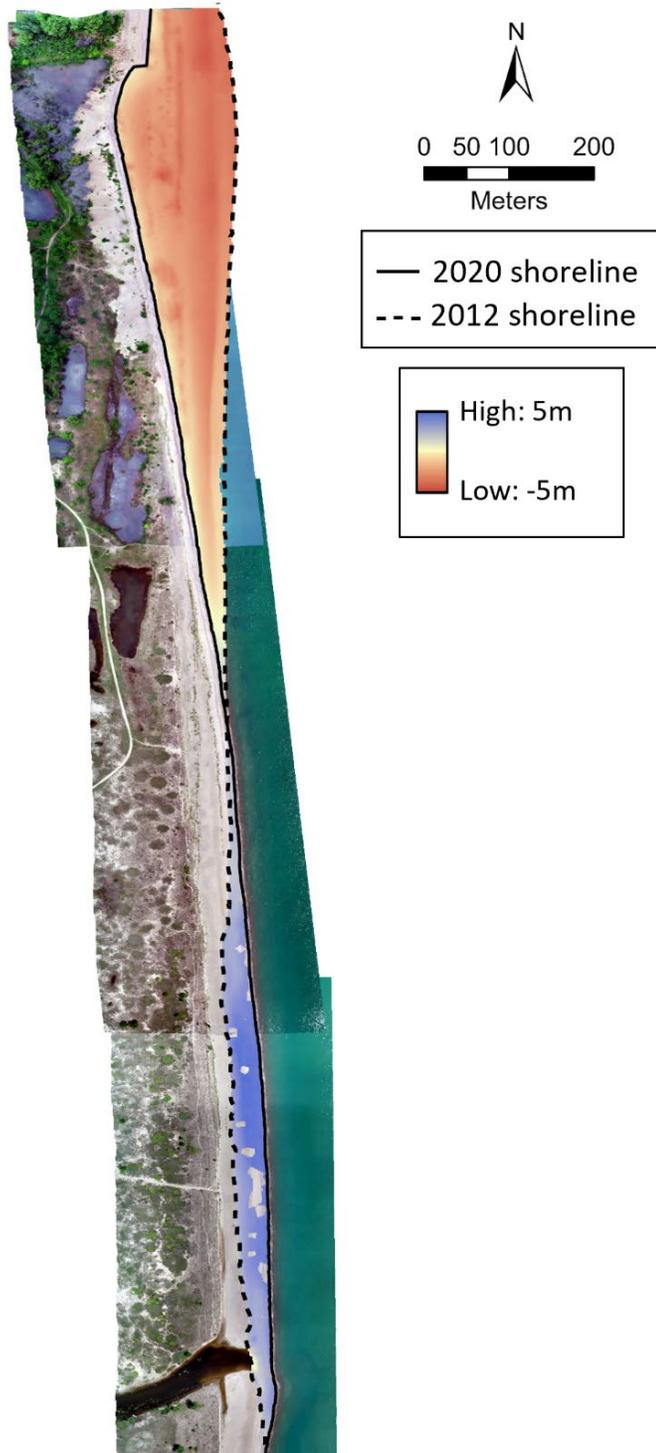
**Figure 33** – Geomorphic change model based on 2012 and 2020 LiDAR-derived DEMs, showing the loss of sediment and beach terrains in the north and accretion/progradation of beach terrains in the south of IBSP4-6.
