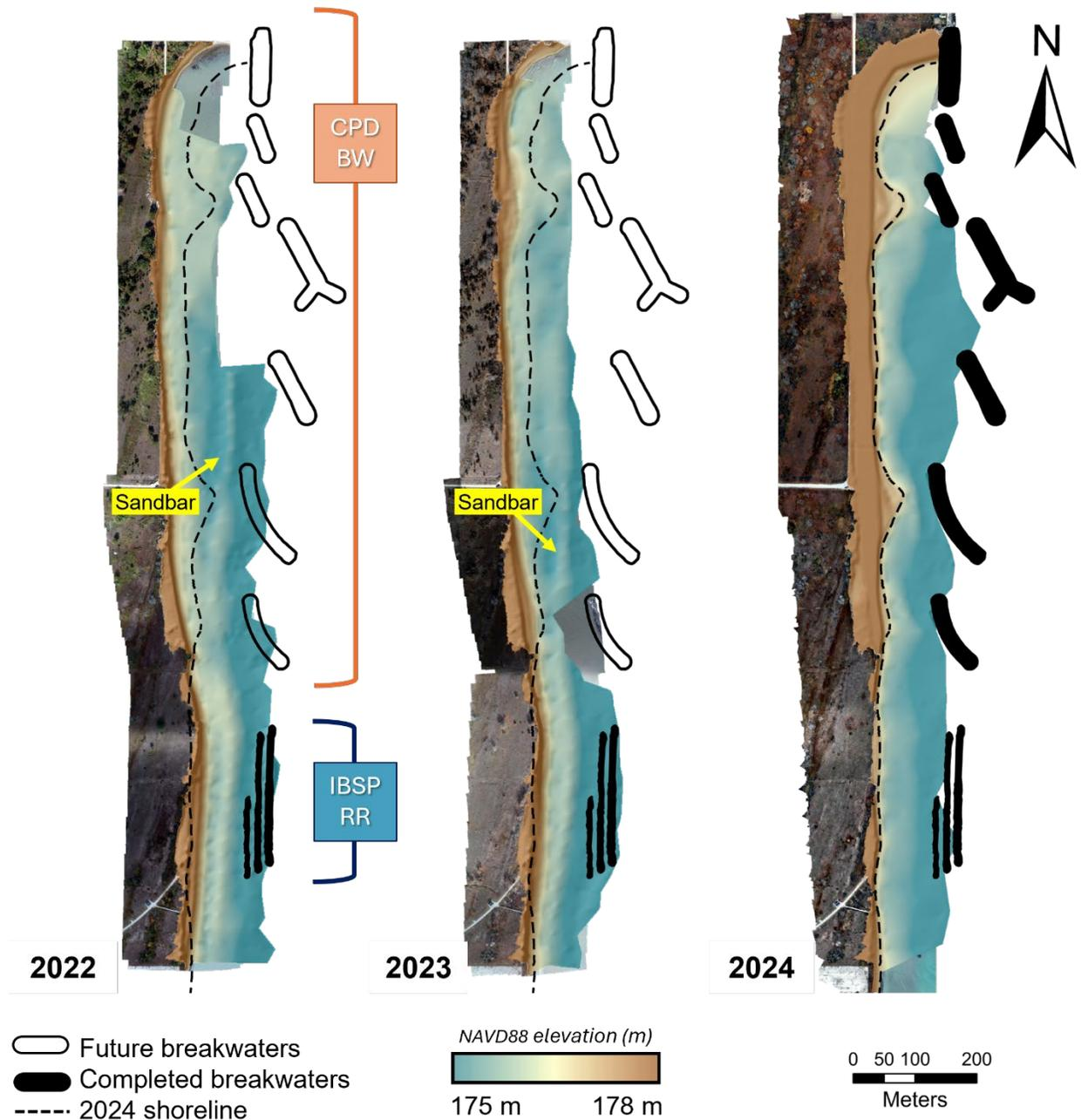
**Figure 31** – Topobathymetric models for IBSP2-3, based on November 2022, 2023, and 2024 ISGS surveys. Submerged rubble-mound breakwaters (IBSP RR) were built in 2022; emergent breakwaters and beach nourishment (CDP BW) was completed in Spring 2024. The absence of a nearshore sandbar in 2024 is noted, along with tombolo formation. The shoreline in the immediate downdrift of the CPD BW site has continued to recede, as evidenced by 2022 (pre-construction) and 2024 DEMs.
