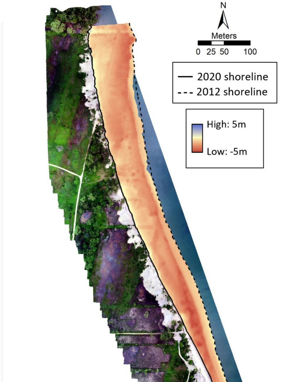
**Figure 24** – LiDAR topo-bathymetry data from 2012 and 2020 show how much ridge-plain terrain was lost with lake-level rise. Shown here is the geomorphic change model for the area between 2012 and 2020 shoreline positions. Little of this volume of sand loss was retained on site as washover fans, portions of which can still be made out along the landward perimeter of the 2012-2020 erosional wedge. Sand was exported from this historically erosive site.
