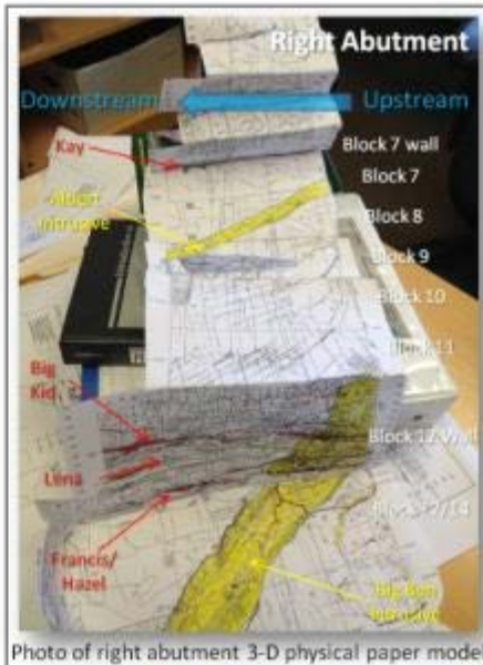
Photo of right abutment 3-D physical paper model
