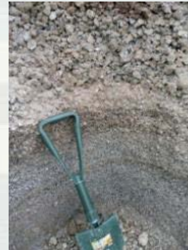
Lapilli tuff (typ.) readily alters to clays, zeolites and consolidates.
